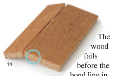
The wood fails before the bond line in this test and many other applications.
