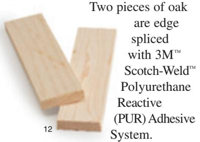
Two pieces of oak are edge spliced with 3M™ Scotch-Weld™ Polyurethane Reactive (PUR) Adhesive System.
