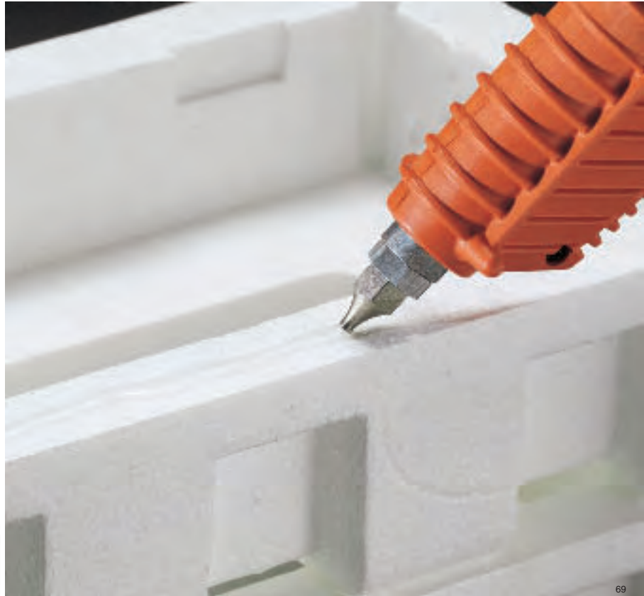
3M™ Scotch-Weld™ Hot Melt Applicator EC can be used with 3M low temperature (265°F/129°C) adhesive to effectively bond heat-sensitive substrates such as styrene foam.
