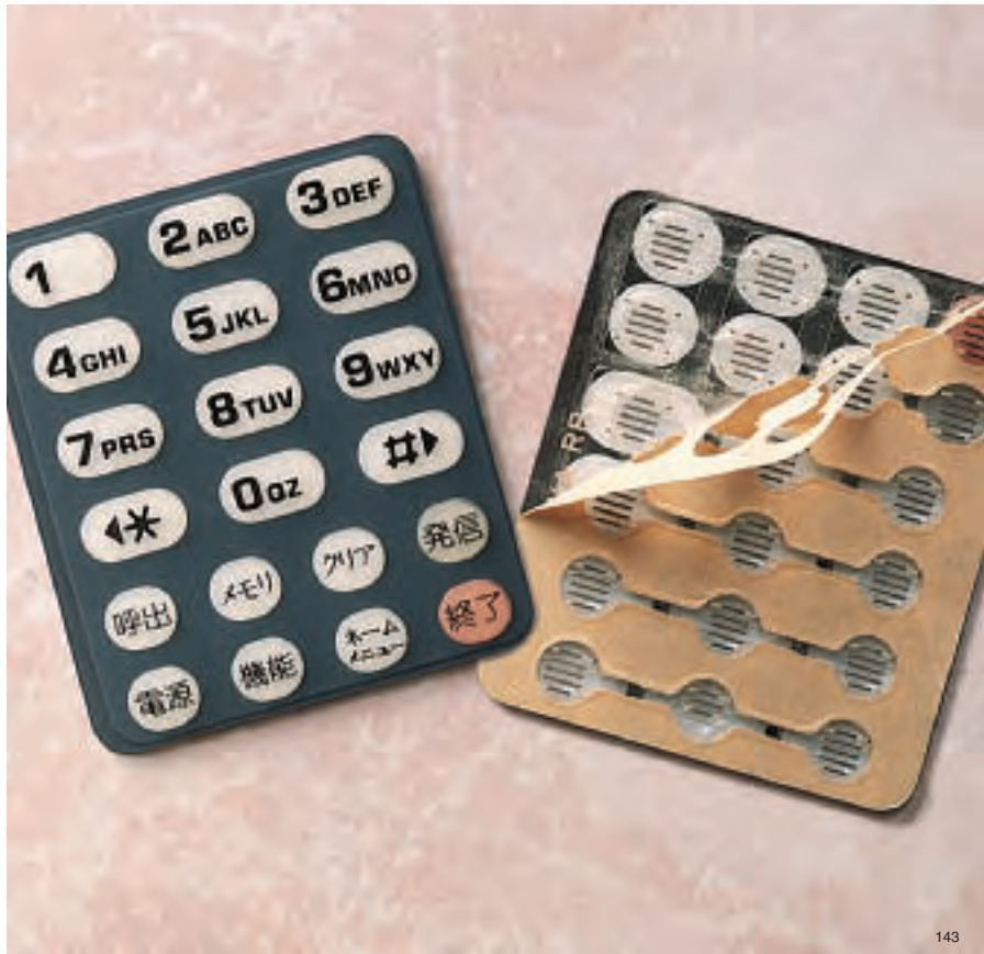
3M™ Double Coated Tape 9731, features differential adhesive for silicone rubber keypad assembly. The silicone adhesive side adheres to the silicone rubber keypad. The acrylic adhesive side adheres to a plastic base.
