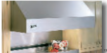
In range hood assembly, 3M™ Structural Bonding Tape replaces spot welding. The tape provides the strength of welding while sealing edges and preventing leaks. Tape also eliminates refinishing the steel after welding.
