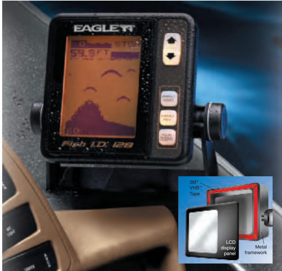
3M™ VHB™ Tapes bond the lens on contact in a fish finder and seal against water, moisture, salt, and more. Bonding power eliminates mechanical fasteners for a smooth, clean surface. Viscoelastic properties help absorb shock and vibration for bond reliability.
